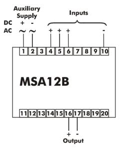
Connections vary with input and output combinations. Individiual connection diagram are supplied with each instrument.
