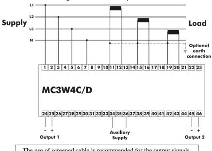
The use of screened cable is recommended for the output signals.
